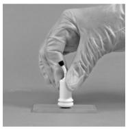
Before activation shake the GCP CAPSULE to loosen the powder. For activation press the plunger on a plane surface to the end into the capsule.
