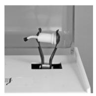
Insert the GCP CAPSULE into a mixer (or an amalgamator), close lid and mix immediately for 10-15 seconds (about 4300 oscillations / min).
